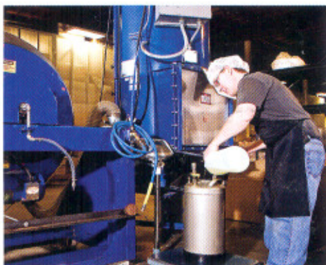
A variety of natural flavours can be added to the tea via an internal spray system. Choice Organic also uses the spray system to neutralise the flavours between batches.
