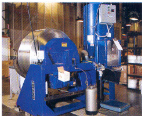
A variety of natural flavours can be added to the tea via an internal spray system. Choice Organic also uses the spray system to neutralise the flavours between batches.
