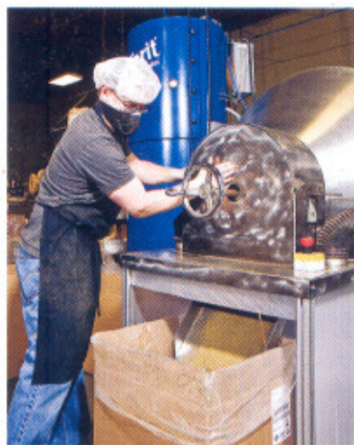
The mixer is self-emptying, resulting in total discharge and no waste.
