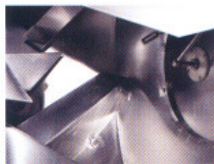
Mixing flights produce a tumble-turn-cut-fold mixing action that yields 100% batch uniformity in less than three minutes.
